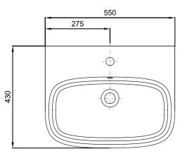
Sizes detailed could have a variation of about +/-5 % due to the changes to material characteristics during the firing processes. Exact measurements for individual installations can only be taken from the finished ceramic
